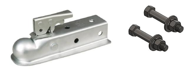
This coupler is to be installed on any 2" wide steel hitch tounge. Use included hardware to secure to the hitch tounge. Some hitch tounges may require the drilling of two 1/2" dia, holes prior to installation.
